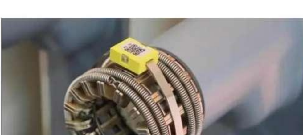
● Installed on Moving Contact of Circuit Breaker
