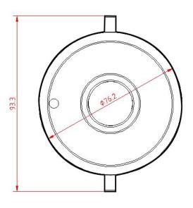
**Installation notes**: the product is easy to install and is embedded. The installation hole size of the sensor is  $\psi$ 58mm. During installation, the product is fixed by the leaf springs on both sides. KNX bus is connected by the bus terminal and other modules.
