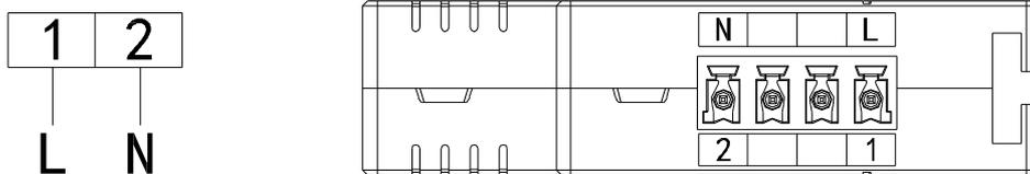
Auxiliary power supply (AC/DC 220V)
